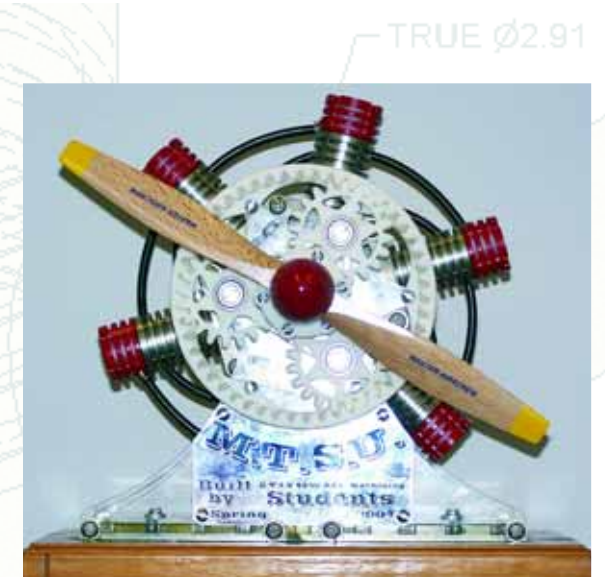
Air motor (a student project in CAD/CAM)
